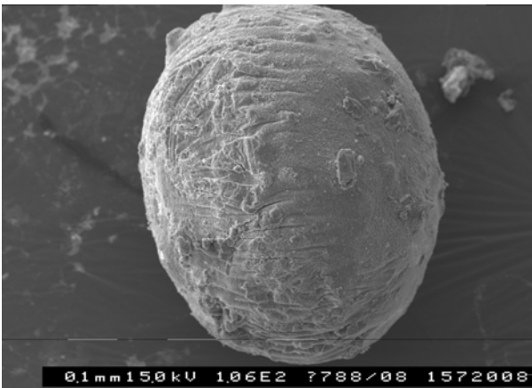
Fig. 7. SEM image of microcapsule (MCF12) shape & size (600 μm)
